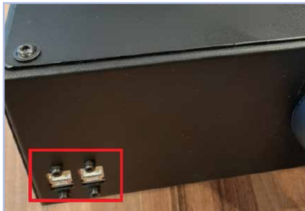
Fig. 6: Tap off box - external DIRIS Digiware connectors.
