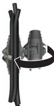
Step 5: Integration of the residual CT in the accessory
