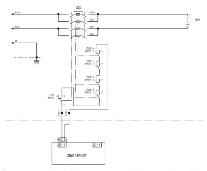
This option enables Q20 to be opened following an emergency shutdown or a slow discharge.
