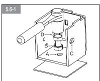
Each foot has a floor fixing hole (labelled A: ø 13) and welded nut for level adjusting (labelled B: screw THM 12 not supplied).
