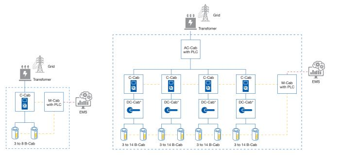
Power connection Power management by PLC Connecting to external EMS Provided by Socomec
