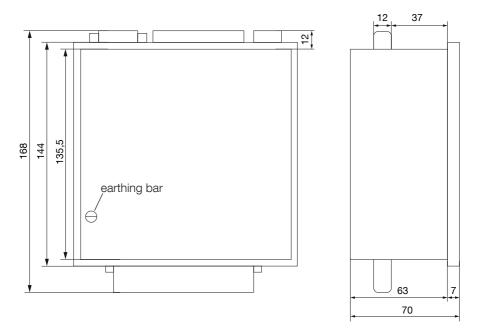
**DANGER!** The rear of the COSYS P to be enclosed in the cabinet or control cabinet has an IP20 degree of protection. Always provide protection against accidental contact with live parts and install the controller in a suitable enclosure to prevent the ingress of dust and liquids (e.g. control panel or distribution panel).
