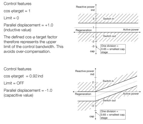
In this case, the cos  $\phi$  target factor represents the lower limit (more inductive) of the control bandwidth. During regeneration, the lower limit (more inductive) represents a cos  $\phi$  target factor of 1. This means that there is no inductive reactive power when power is supplied.
