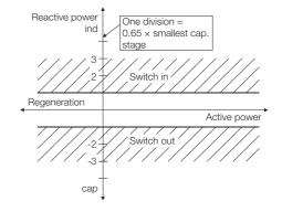
If the system is operating in the band shown, no switching is activated.
