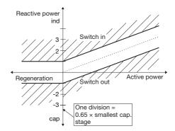
The diagram above shows how the COSYS P acts during regeneration (mains supply). The "elbow" in the band (characteristic line) is not reflected in the regeneration quadrants. Instead, the band extends laterally from the point where it intersects the reactive power axis (Y-axis).
