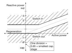
The range of system limits can be set between -2 and +2 in increments of 0.5 and can be disabled. Setting the limit to 1 and the cos  $\phi$  target factor to 1.00 has exactly the same effect as the parallel displacement described above. If the cos  $\phi$  target factor is not set to 1, the control curve shows a characteristic breakage, as shown in the example above.
