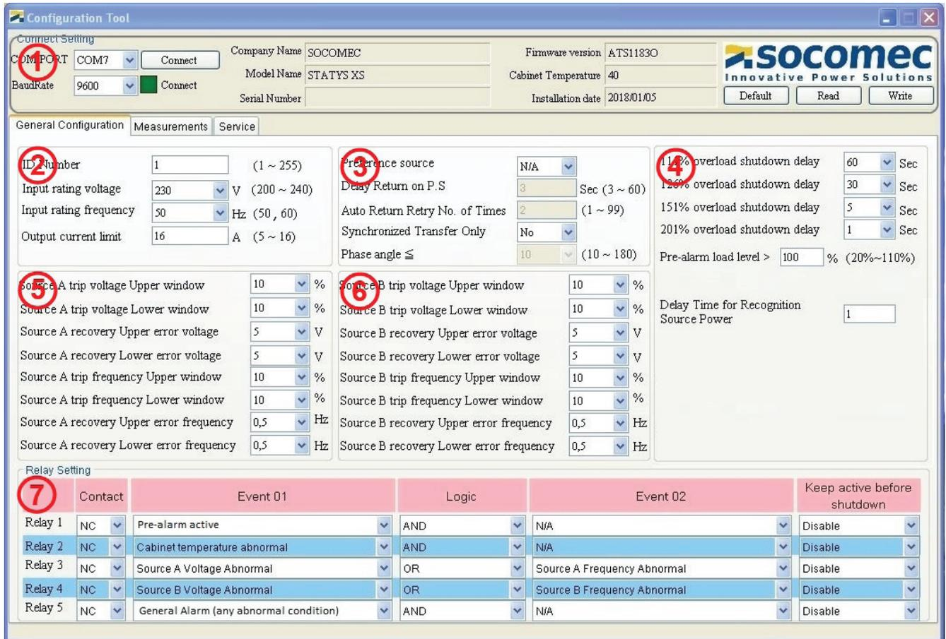
**1** Connect Setting: COM PORT (COM7), BaudRate (9600), Connect button, Company Name (SOCOME), Model Name (STATYS XS), Serial Number, Firmware version (ATS11830), Cabinet Temperature (40), Installation date (2018/01/05), Default, Read, Write buttons.
