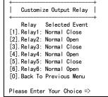
Once the configuration is complete **SW2** MUST be switched to the ON position to apply the new settings. Switch **SW2** back to the OFF position to reset to the default settings.
