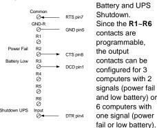
Note: All of the computers must have the same earth ground potential. Connect all of the computers input power to the same UPS.
