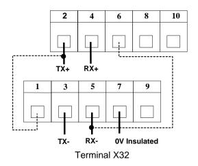
2.3. Connecting the MODBUS/JBUS® link to Power LTMs
