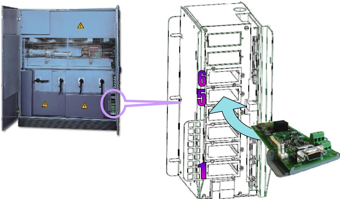
The « Com-Slots » integrates all communication interfaces, and it is located at the bottom of the UPS, on the right side.
