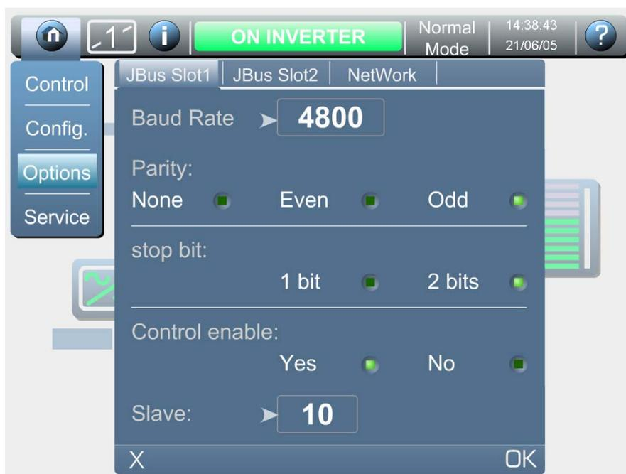
JBUS/MODBUS 1 settings are linked to the interface located in slot 5.
