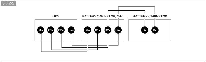
Close the battery bridge circuits according to the diagram on the inside of the door.
