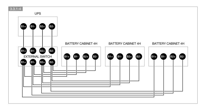
Close the battery bridge circuits according to the diagram on the inside of the door.
