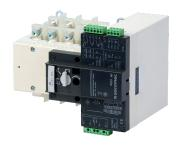
They enable the on-load transfer of two three-phase supplies via remote volt-free contacts, from either an external automatic controller, using pulse logic, or a switch. They are intended for use in low voltage power supply systems where a brief interruption of the load supply is acceptable during transfer.
