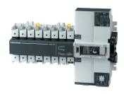
ATyS d M devices are 2 pole or 4 pole transfer switches that are remotely controlled using volt-free contacts from an external controller. They are modular products with positive break indication. They are intended for use in low voltage power supply systems where a brief interruption of the load supply is acceptable during transfer.
