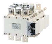
SIRCOVER products are manually operated transfer switches with positive break indication, for overlapping contact switching (I-I+II-II). This combination of three interlocked load break switches provides bypass to an UPS or other devices when sources are synchronised and the UPS is in static bypass mode.
