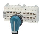
SIRCO VM1 are 3 or 4 pole modular manual transfer switches with visible breaking. They provide on-load transfer between two sources for any low voltage power circuit, as well as safety isolation. Other applications include source inversion (e.g. to change the direction of a motor) or grounding/earthing.
