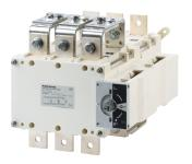
SIRCOVER products are manually operated transfer switches with positive break indication. This combination of three interlocked load break switches provides 3+6 or 4+8 poles for bypass applications.
