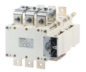
SIRCOVER products are manually operated transfer switches with positive break indication. This combination of three interlocked load break switches provides 3+6 or 4+8 poles for bypass applications.
