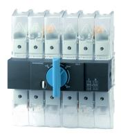
SIRCO M are manually operated 3 or 4 pole modular transfer switches with positive break indication. They provide on-load transfer between two sources for any low voltage power circuit, as well as safety isolation. Other applications include source inversion (e.g. to change the direction of a motor) or grounding/earthing.
