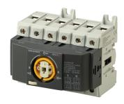
SIRCO M are manually operated 3 or 4 pole modular transfer switches with positive break indication. They provide on-load transfer between two sources for any low voltage power circuit, as well as safety isolation. Other applications include source inversion (e.g. to change the direction of a motor) or grounding/earthing.
