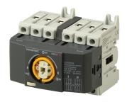
SIRCO M are manually operated 3 or 4 pole modular transfer switches with positive break indication. They provide on-load transfer between two sources for any low voltage power circuit, as well as safety isolation. Other applications include source inversion (e.g. to change the direction of a motor) or grounding/earthing.
